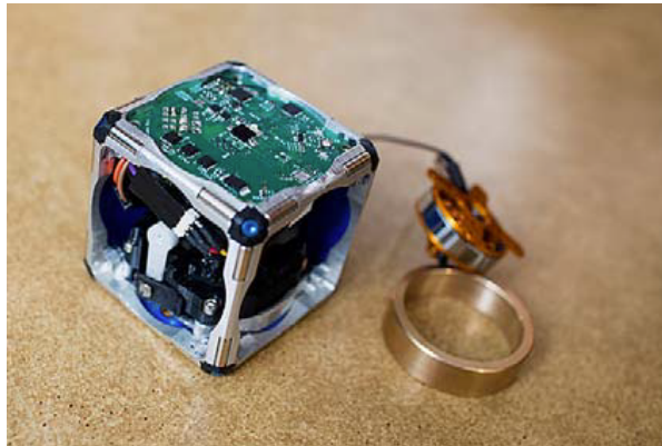
Fig. 1 The M-Block with its innards exposed and its flywheel
