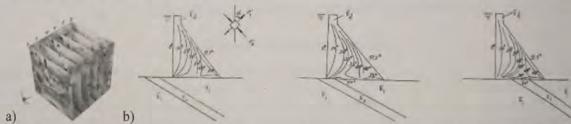
Figure 2: a) Isochromatics in a 3D printed specimen of concrete tested by stress freezing photoelastic method [3], b) Isoclines in the tested gravity dam for the three considered positions of a discontinuity in the foundation soil [4]
