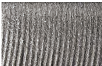
Fig. 7. Cut surface generated in abrasive water jet cutting of aluminium alloy
