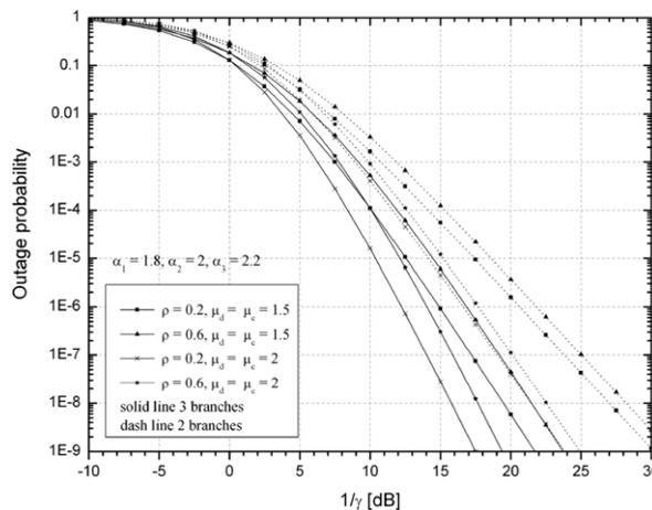
**Fig. 5.1.** Outage probability versus  $1/\gamma$ .
