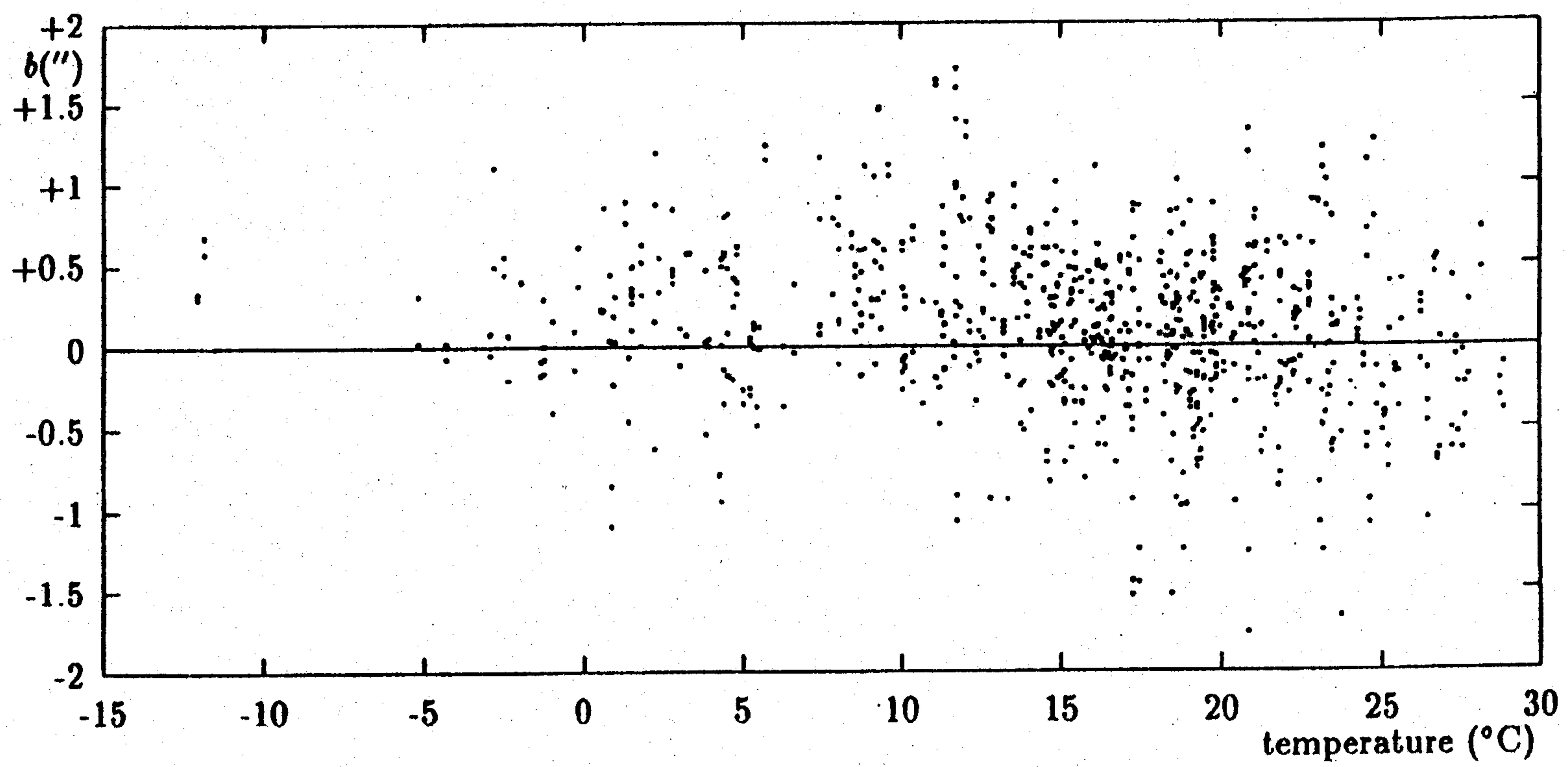
**Fig. 2.** 754 values of BVC flexure versus temperature.
