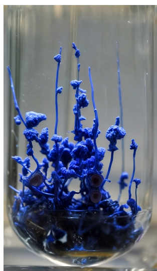
Figure 1: Silicate chemical gardens grown under normal gravity conditions. The morphological aspect observed is typical of chemical gardens obtained by the seed growth method.
