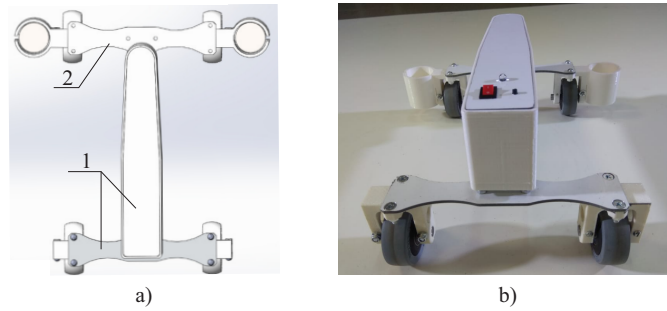
FIGURE 11. a) 3D model and b) picture of the full-scale specimen of the roller racer
