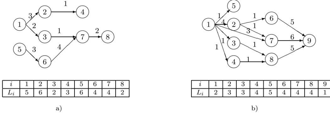
Figure 2: a) *sih91* - Task graph example from [25];b) *kwok* - Benchmark task graph from [11]
