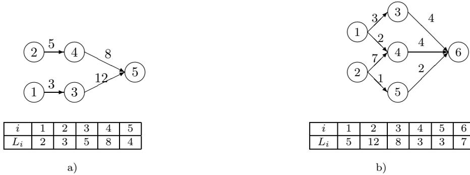
Figure 1: a) *counter* - Task graph example from [3]; b) *test* - Task graph with 6 nodes
